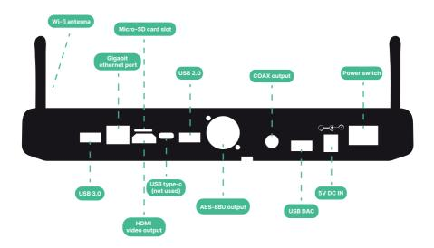
**WI-FI ANTENNAS**: to ensure optimal wireless performances on 2.4/5GHz network, connect the provided double antennas.
